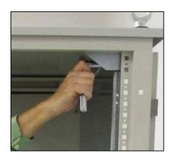
E) Secure the panel to the top panel studs.
